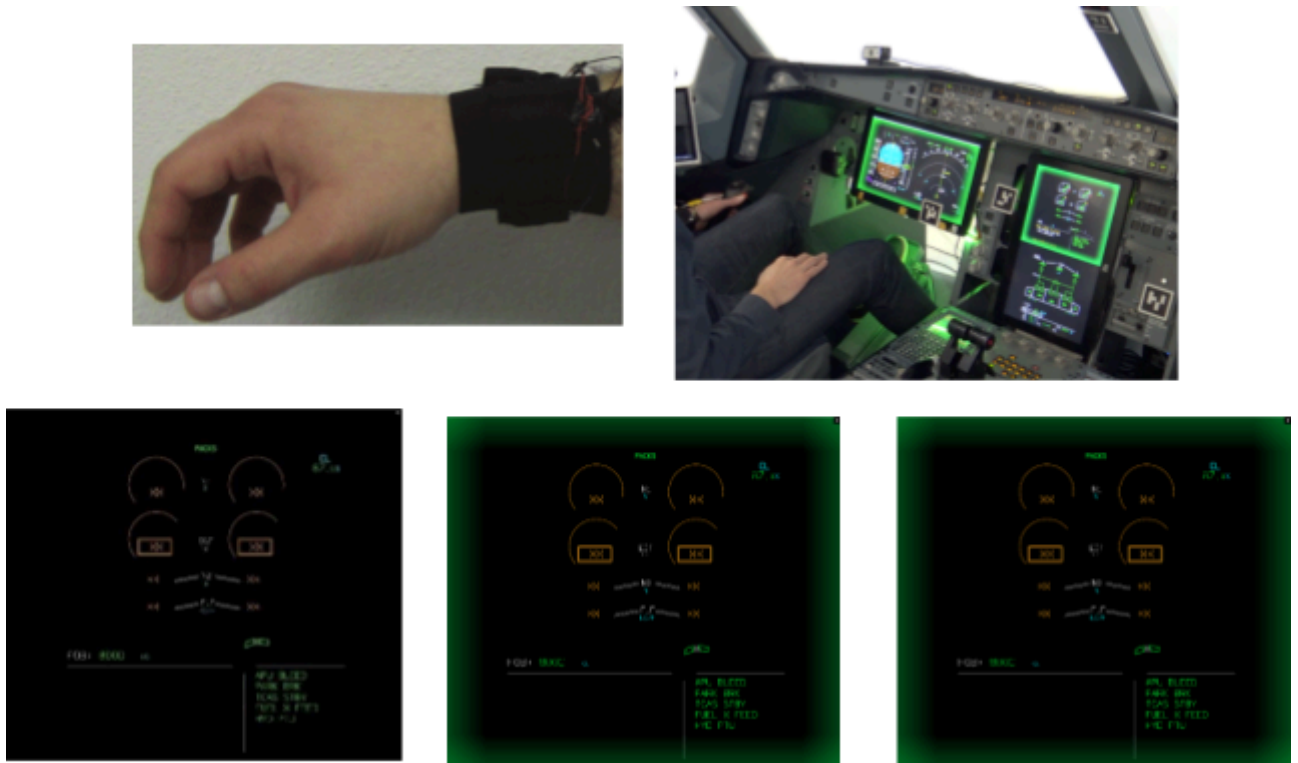
Figure 4: Stress regulation function HMI. Green light emanation around displays and haptic wristband.
