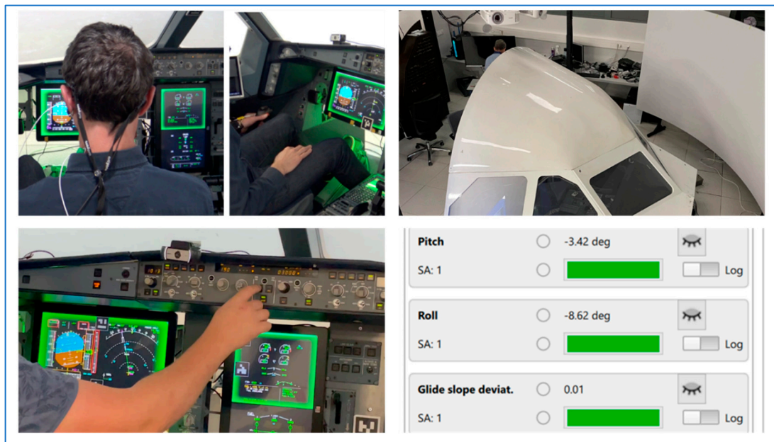
Figure 4. Images from HAIKU Use Case 1 simulation (FOCUS simulation development at Ecole Nationale Aviation Civile (ENAC) Labs, Toulouse, France) [10], showing the cockpit simulator (top right), a pilot in the cockpit being supported after startle (top left), an extract from the eye tracking analysis of key parameters the pilot may need to focus on (bottom right), and highlighted directed situation awareness (vertical speed) on the primary flight display (PFD) (bottom left).
